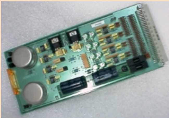
▼ VX-2086 fitted with input transformers
